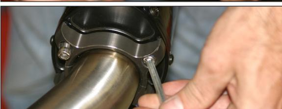
25. Install TBR muffler assembly to bike, use supplied barrel clamp at joint and rubber lined muffler clamp
