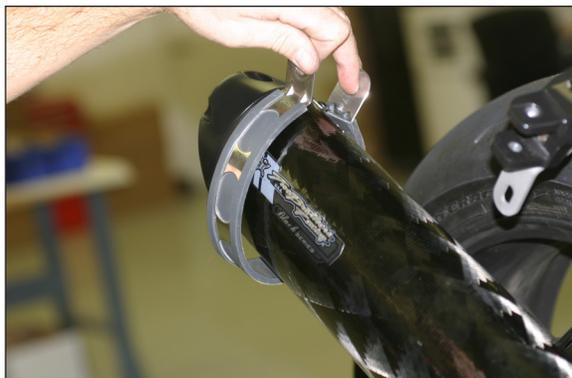
26. Loosely attach to bracket using the supplied bolt with decorated washer and spacer using the supplied 8mm flange
