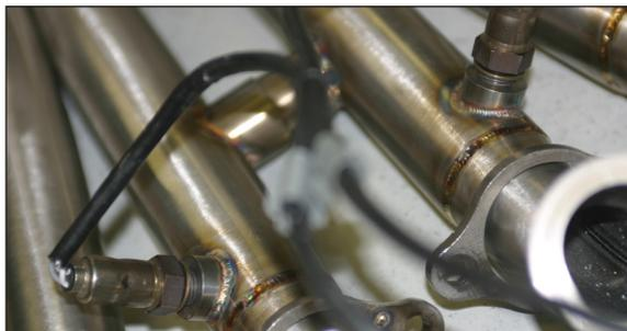
17. Install header assembly making sure to re-use the OEM gasket between header and cylinder head.
