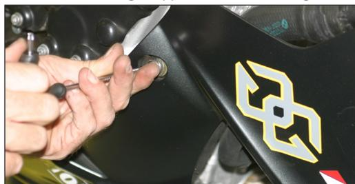
4. Carefully remove crossover servo cable. Do not turn servo wheel (damage may occur if you do). Keep servo plugged in. This servo is located on left side of motorcycle at the lower front of fuel tank.
