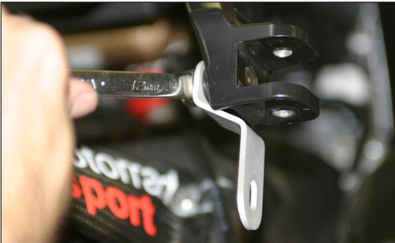
24. Attach TBR muffler to supplied slip-on tube using the provided four 6x20mm socket head cap screws, washers and thread-lock.
