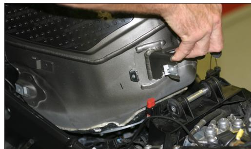
6. Remove both cables from servo carefully. Do not turn servo, the servo must stay plugged in and on motorcycle.
