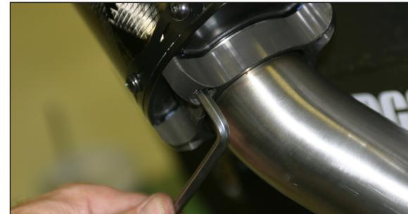
27. Align muffler and securely tighten the x-ring bolts in a cross pattern.
