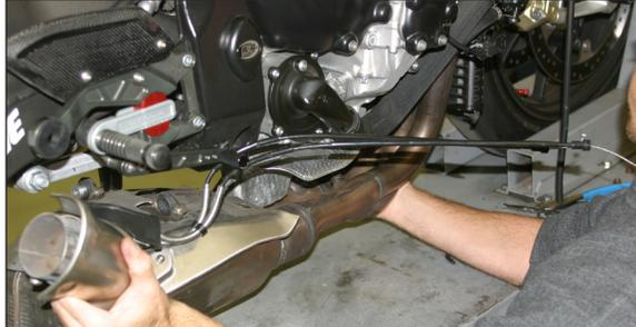
16. Install left and right O2 sensors on header prior to install.
