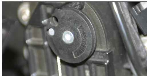
5. Remove/lift fuel tank to access second servo, located under rear of fuel tank.
