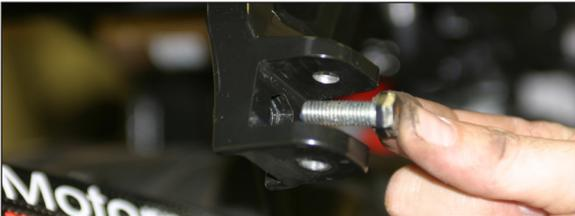
23. Install supplied muffler mounting bracket to newly installed bolt and secure in place with 8mm flange nut.
