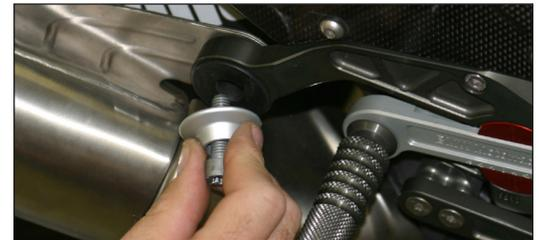
8. Loosen joint clamp and remove muffer assembly.
