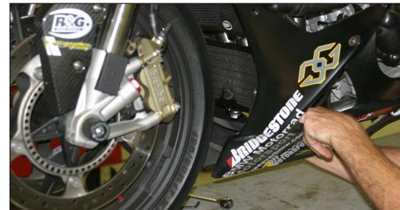
29. Re-install bodywork and check to be sure there is clearance between exhaust tubing and all bodywork.
