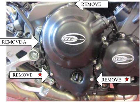
In this kit there should be: 1x Engine Case Cover (ECC0163) 4x M6 x 40mm long button head bolts 2x M6 Washers 1x 'P' clip
