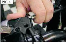
PIC 5 nylon cable anchor out of the stock lever freeing the cable. Remove the OEM nylon
