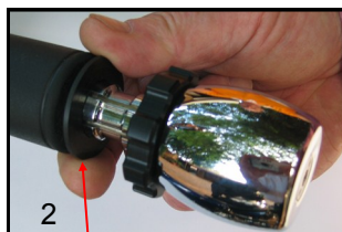
2 Thrust Washer—recess Facing Throttle Sleeve
