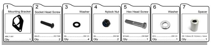
**Step One:** Bolt the ignition to the mounting bracket (#1) using the screws washers and bolts provided (#2,3,4). Remove the OEM upper right hand side frame bolt. Use the spacer washer and bolt (#5,6,7) to attached the ignition bracket to the motorcycle.
