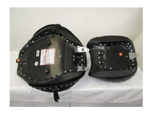
3. Remove the center bracket from the fender. If installing a solo alone, these bolts will be used to mount the Mustang solo.
