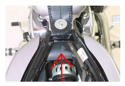
2. Ensure the rear brackets are aligned so they will slide under the fender studs.
