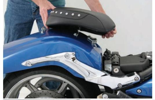
2. Align and install two bolts to secure front of rear seat to fender bracket.
