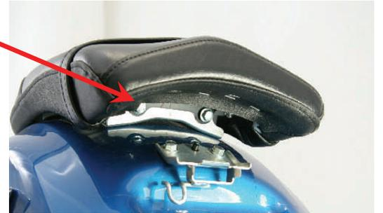
3. Then pull rear seat forward and off of its fender bracket.
