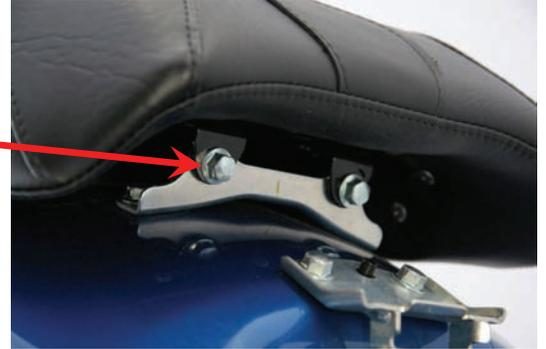
3. Tilt front of driver's seat up and push rear of seat onto fender bracket. Then align front bracket with slot for latch and push front of seat down firmly to engage latch.
