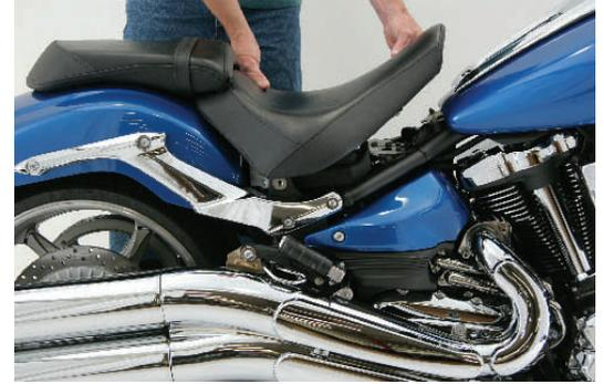
2. Remove the two bolts at the front of the rear seat.
