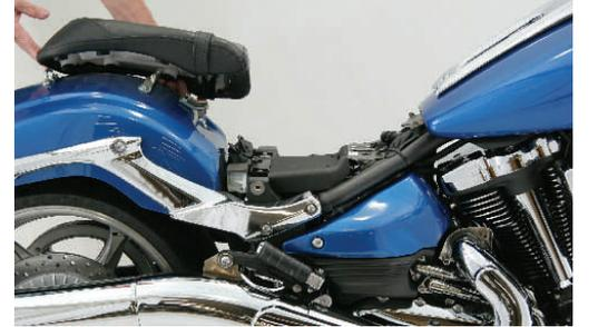
4. In preparation for installation of Mustang seat, locate all four mounting points:
