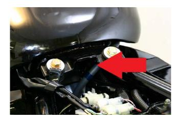
3. Align the solo's rear bracket with the fender mount, position a white nylon washer between the bracket and the fender, and secure with the stock bolt.
