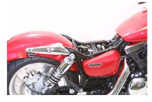
4. Secure the rear bracket to the fender with the stock acorn nut.
