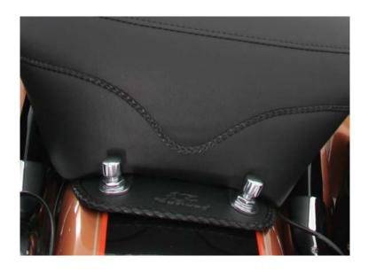
5. Place the nylon shoulder washers (1999-2007) or flat washers (1997-1998) on the fender studs and then put the rear mounting tabs over the studs.
