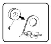
5. Install (No. 5) *ALS-046*, aluminum spacer in the front side of (No. 4) *Z1023*, rubber grommet and install (No. 6) *ALS-054* for *Husqvarna OR ALS-057* for *KTM*, aluminum spacer in the back side of (No. 4) *Z1023*, rubber grommet as shown below.
