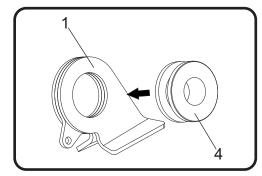
2. Install (No. 11) *ALS-043*, aluminum spacers into (No. 4) *Z1023*, rubber grommet as shown.
