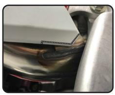
Before starting motorcycle, check for proper clearance between new exhaust system and rear suspension (i.e. tire, swingarm, brakes, rear shock, and etc.) If any problem is found, please carefully follow through the installation steps again. If problem still persists, please call Yoshimura Tech Department at (800) 634-9166 / in CA (909) 628-4722.
