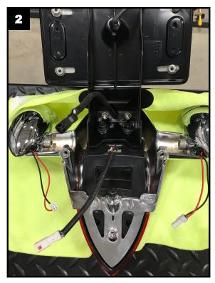
4. Remove the 2 bolts and spacers securing the stock license plate mount to the taillight housing. Retain the bolts and spacers as they will be used for reassembly. Refer to Picture 3.
