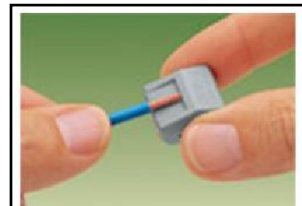
Strip wire 9-10 mm. Use wire gauge on bottom to verify.
