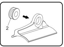
Install (No. 5) ALS-047 for Husqvarna OR ALS-056 for KTM, aluminum spacer in the backside of (No. 2) Z1023, rubber grommet and install (No. 3) ALS-046, aluminum spacer in the frontside as shown below.
