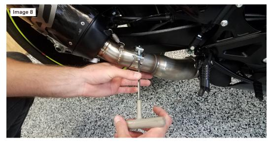
Before you run the bike, clean off all fingerprints and dirt, as any oily residue will etch the metal and become somewhat permanent when the system gets hot. Run the bike and enjoy. Check for gaps or leaks. After 50 to 100 miles, recheck all fasteners for tightness.
