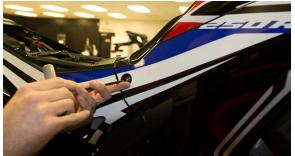
3. Loosen and remove the exhaust bracket bolt and clamp bolt.
