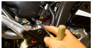
Using the included 8 x 75mm bolt, spacer, and 8mm nut – install the muffler with muffler clamp to the TBR slip tube. NOTE: Be sure to put the spacer in place on the bike before sliding the bolt through.
