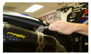
9. Before you run the bike, clean off all fingerprints and dirt, as any oily residue will etch the metal and become somewhat permanent when the system gets hot. Run the bike and enjoy. It is normal for some white smoke to appear the first time you start the bike. This is packing/manufacturing oil from inside the pipe burning off. Check for gaps or leaks. If you find a leak, a little high temperature silicon sealant should fix it. After 50 to 100 miles, recheck all fasteners for tightness.
