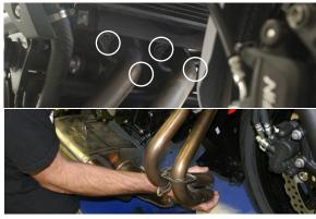
6. Attach supplied muffler mounting bracket to the three rubber mounting supports. Use supplied nuts and bolts.
