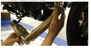
Install TBR Muffler assembly using supplied barrel clamp at header joint.
