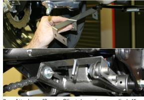
Attach muffler to Slip tube using supplied 45mm springs.
