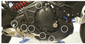
Remove the right foot rest assembly to access muffler mounting bolts.
