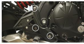
Remove muffler mounting hardware.
