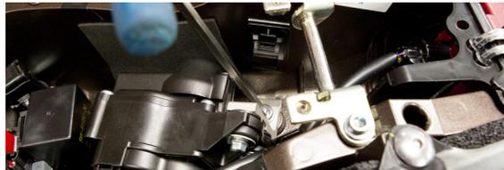
10. Remove servo cover and remove servo cables. Be sure not to damage servo during the process.
