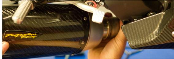
19. Slide rubber lined muffer clamp over muffer and attach to previously installed bracket using the supplied 8x20mm socket head cap screw and 8mm flange nut.
