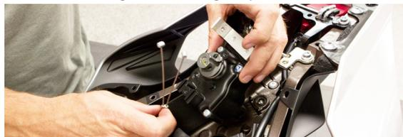
11. Remove cables from motorcycle by pushing cables in from the top and out through the bottom of tail section.
