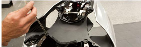
9. Remove servo retaining bolt and lift servo up to access servo cover screws.
