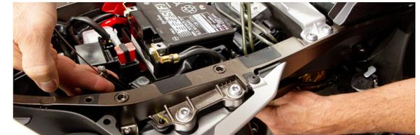
12. Re-install servo motor and secure in place with retaining bolt. The servo motor must be connected and functions properly to keep engine light off.
