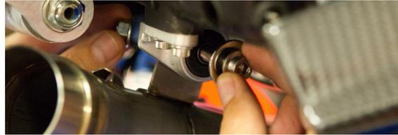
17. Attach supplied TBR muffer mounting bracket using the OEM bolt and supplied 8mm nut to OEM mounting point behind rear set.
