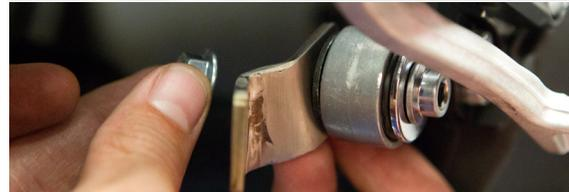
18. Attach TBR slip muffer assembly to y-pipe using supplied springs.
