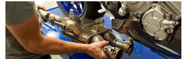
16. Install TBR y-pipe by using the supplied t-bolt clamps, OEM bolt, and supplied 8mm nut on center bracket.
