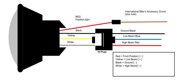
**Note:** The Red (position light or city light) wire is intended for international application where a position light to be illuminated in the headlight while the bike is parked on the street is required.
