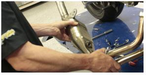
Attach TBR header to motorcycle, be sure the OEM gaskets are between the headed and engine. Use supplied nuts in place of OEM cap nuts.
