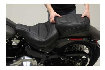
4. Align the rear bracket with the rear fender nut and secure with the supplied Nylock fender screw.
