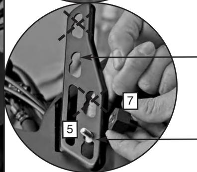
The bushings must be mounted in the lower mount position to avoid interference with mirror.
