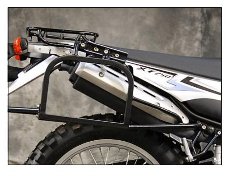
Note pictures are of SU rack, but installation is same with exception SL racks do not have a rear support bumper. Turn signal bracket shape changed, but mount similar.
