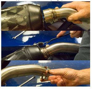
7. Install TBR muffler assembly to motorcycle using the supplied barrel clamp at header joint and OEM hardware.
