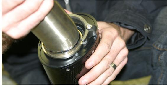
4. Slide a supplied barrel clamp on to each slip tube.
