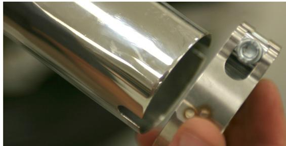
5. Insert the slip tube of each V.A.L.E.™ muffler assembly into OEM head pipe.
