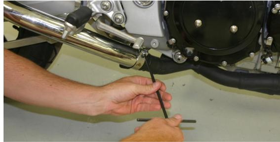
10. Securely tighten the 8x40mm and 8x50mm cap screws.
