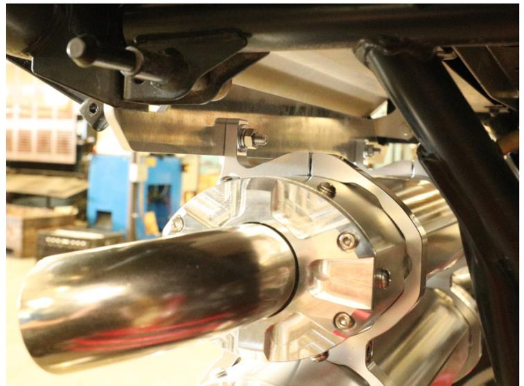
6. Loosely mount mufflers to vehicle.
