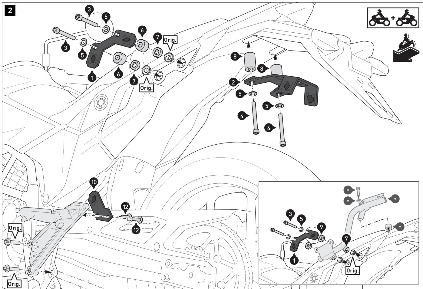
**⚠ NOTE:** The detailed drawing shows the installation of the side carrier with the SW-MOTECH rack. Use the mounting parts included with the rack [-] in combination with the mounting parts shown for the side carrier.
