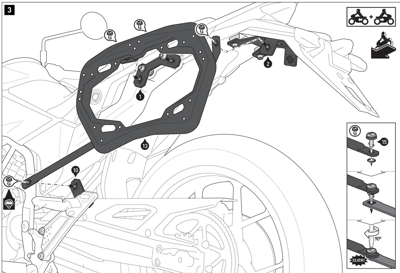
**⚠ NOTE:** SW-MOTECH anti-theft protection is sold separately; mount the anti-theft protection onto **both sides** of the vehicle as indicated.
