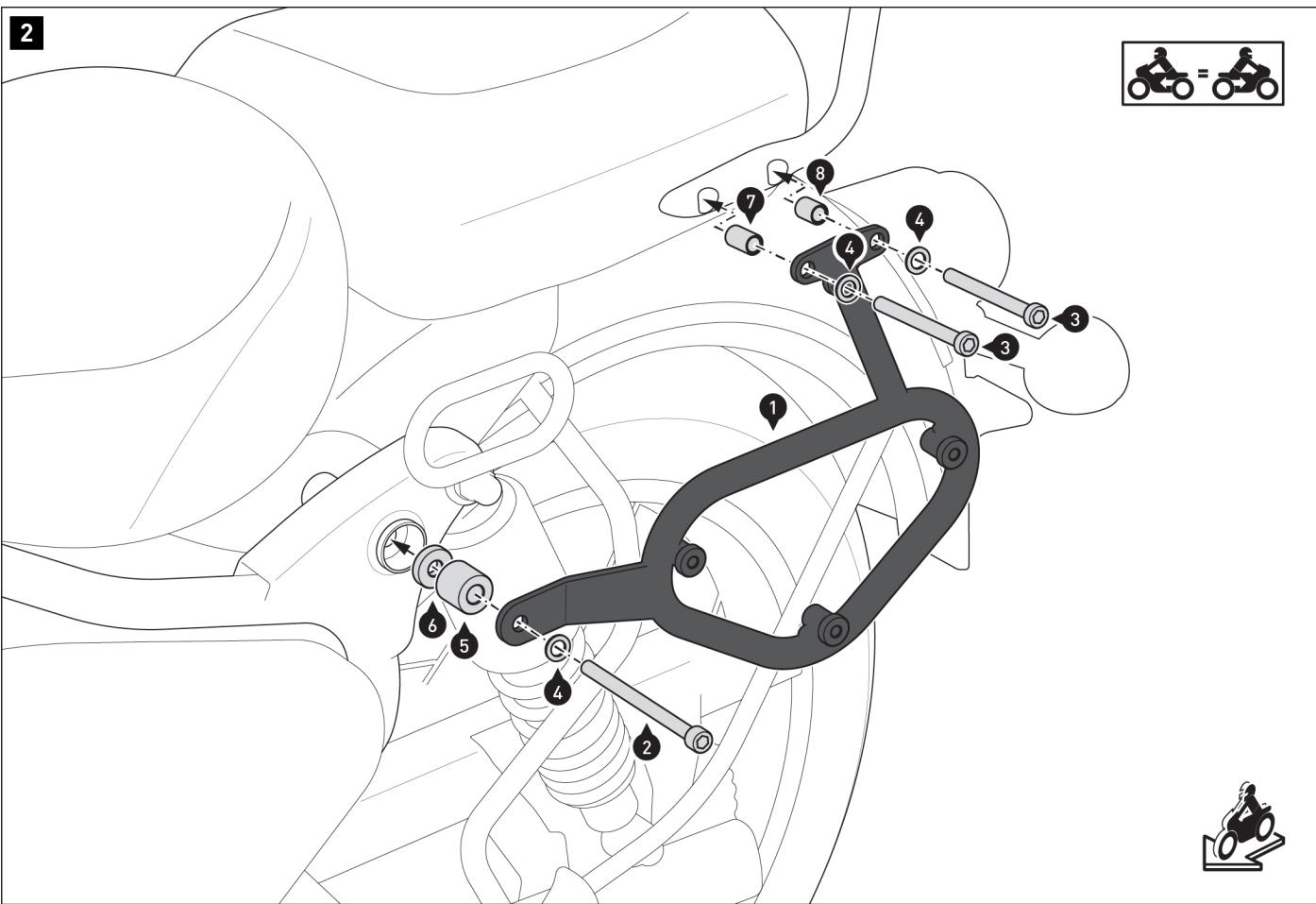
Screw the side carrier (1) to the vehicle.
