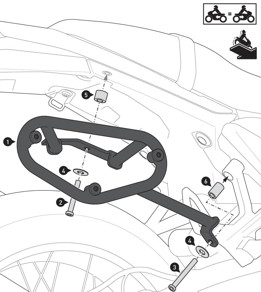
**⚠ NOTE:** The detailed drawing shows the installation of the side carrier with the SW-MOTECH rack. Use the mounting parts included with the rack (1) in combination with the mounting parts shown for the side carrier.
