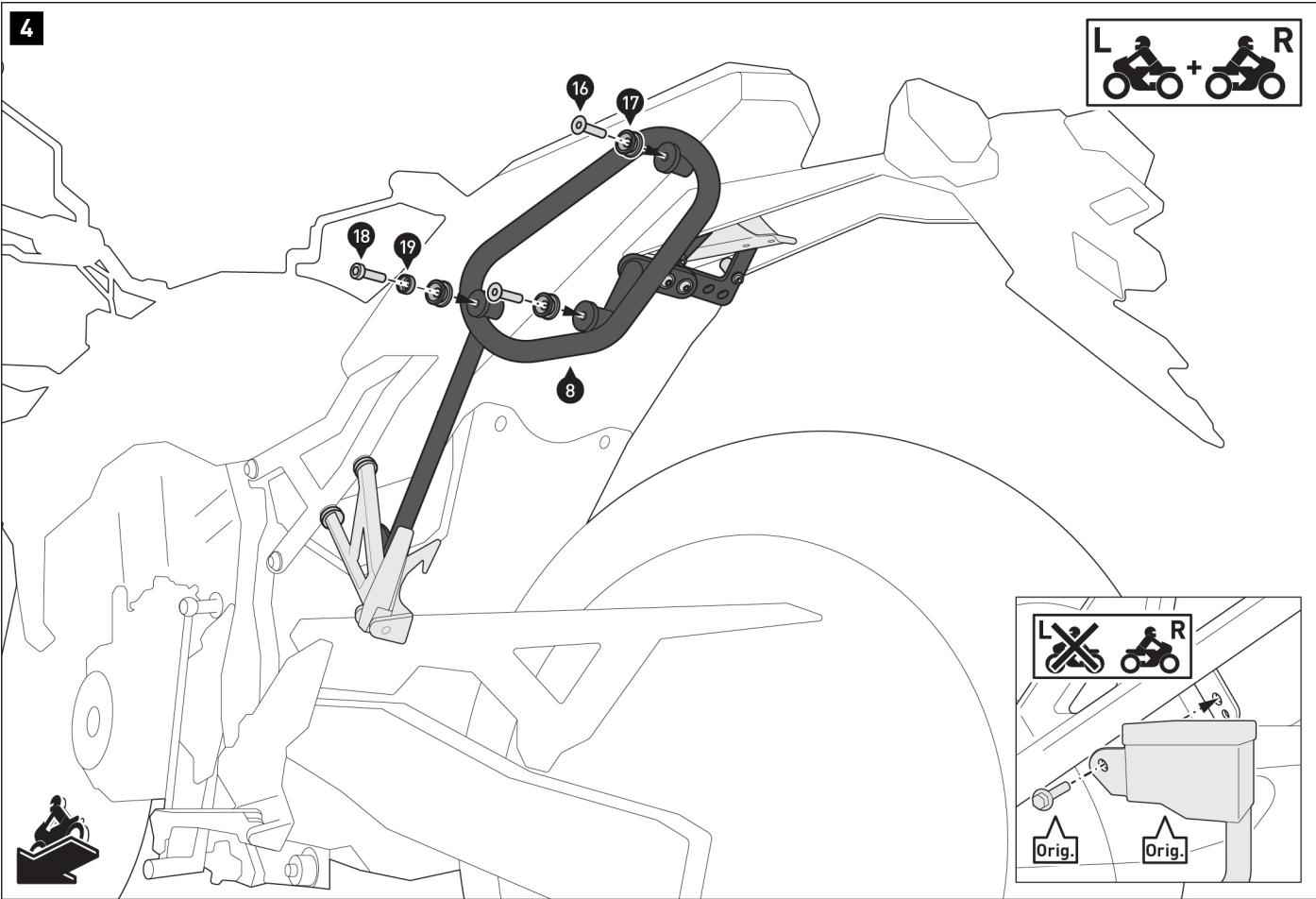
Screw the parts (16) to (19) onto the side carrier (8/9).
