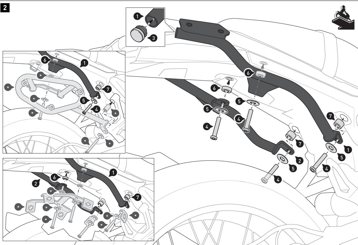
**⚠ NOTE:** The detailed drawing shows the installation of the luggage carrier with the SW-MOTECH **SLC side carrier** (above) and **PRO side carrier** (below). Use the attachments included with the respective side carrier (•) in combination with the attachments shown on the luggage carrier.
