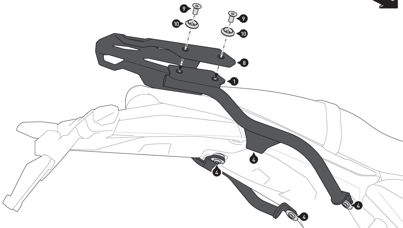
Mount the rack (8) onto the mounting struts (1/2).
