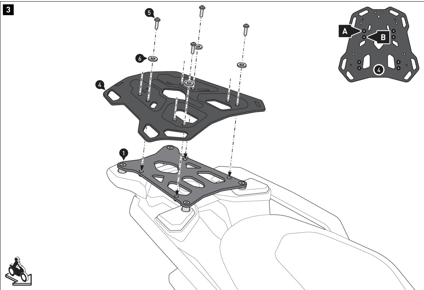
**⚠ NOTE:** Depending on the space available, screw the rack (4) to either mounting position (A) or (B), as illustrated in the detailed drawing.
