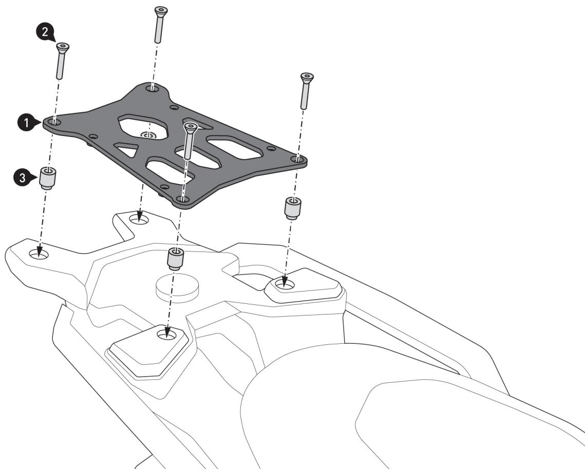
Screw the mounting bracket (1) to the attachment points as indicated.
