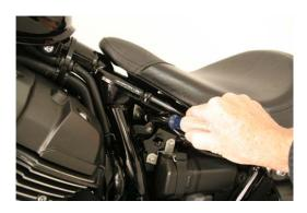
3. Lift the nose of the seat and slide forward to remove the solo seat.
