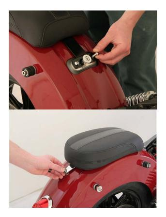
3. Holding the solo seat parallel to the frame, engage the solo seat's rear bracket with the fender stud.
