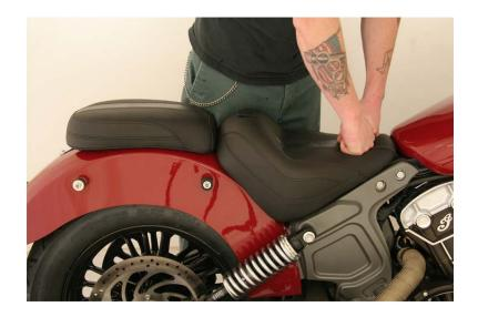
4. Ensure the rubber grommet aligns with and engages the frame stud behind the tank, and press firmly down at the nose of the seat. This is a pressure-fit connection. Ensure the seat is secure before riding the motorcycle.
