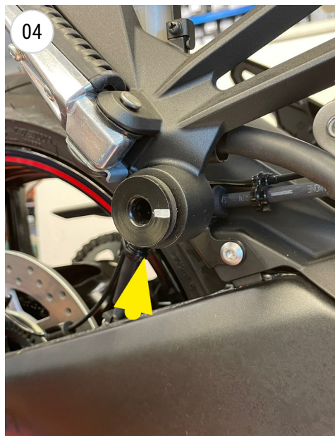
REMOVE THE STOCK SPACERS
