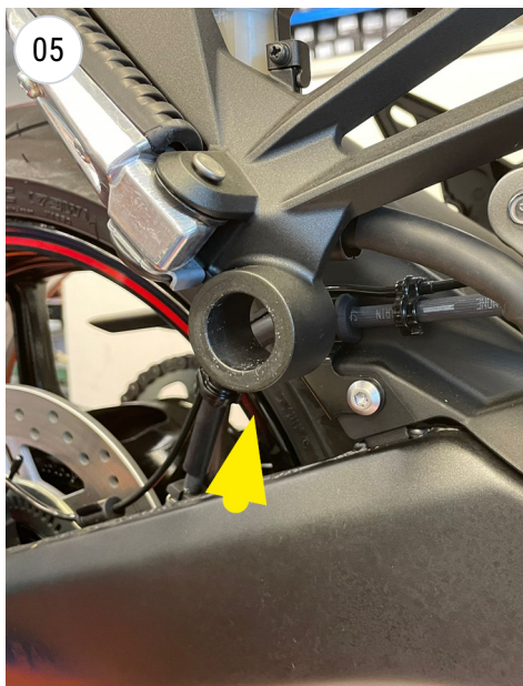
REMOVE THE STOCK SPACERS
