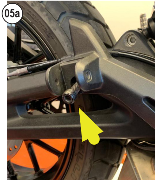
REMOVE THE SCREW AND THE FOOTPEG
