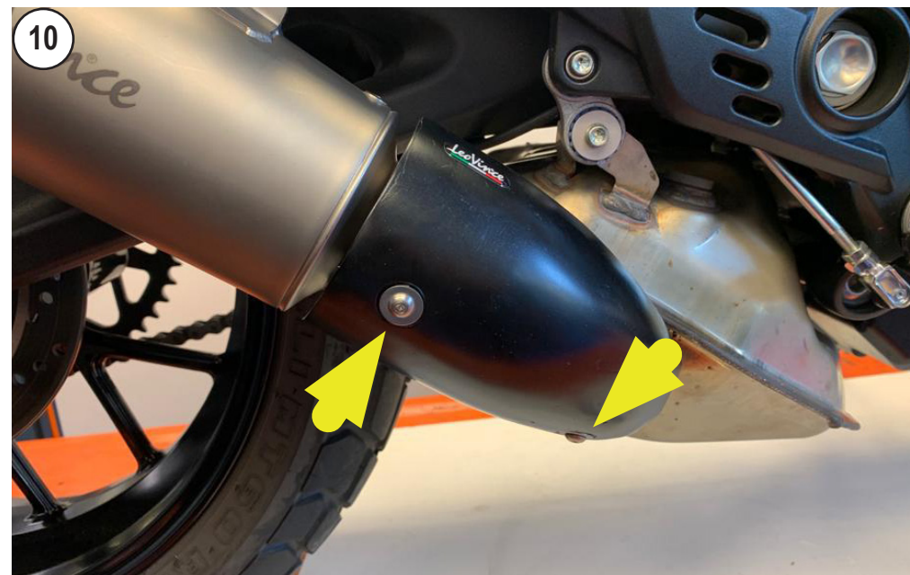
FIT THE CARBON HEAT SHIELD
