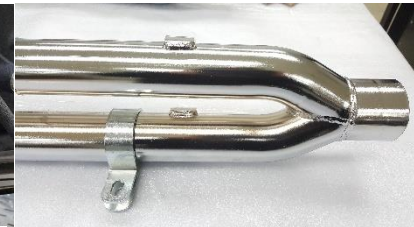
Figure 2.4 Install P-Clamp as shown.
