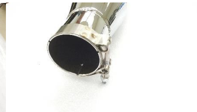
Figure 2.7 Install T-Bolt clamp as shown.
