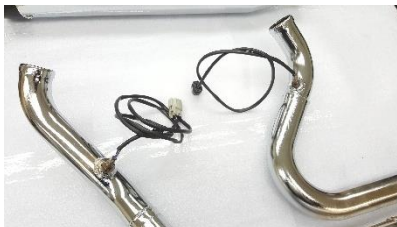
Figure 2.5 Install Oxygen sensors.
