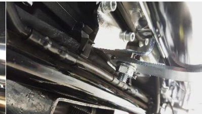
Figure 2.11 Align P-Clamp to mounting bracket.
