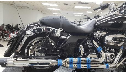
Figure 2.16 Both shields and collector shield installed.
