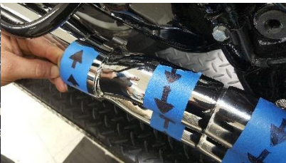
Figure 2.15 Install collector heat shield.
