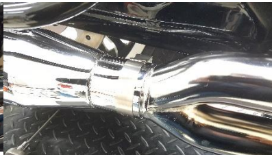
Figure 2.10 T-Bolt clamp faces in and points down.
