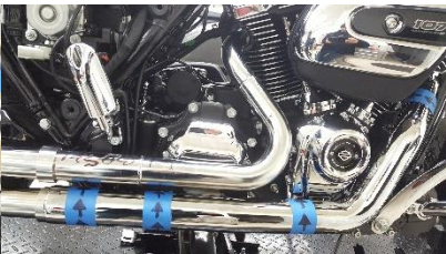
Figure 2.14 Install heat shields.
