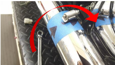
Figure 2.13 Install hose clamps as shown.
