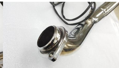
Figure 2.6 Install flanges and retaining rings.
