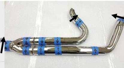
Figure 2.12 Mark center of welded clips with and arrow.
