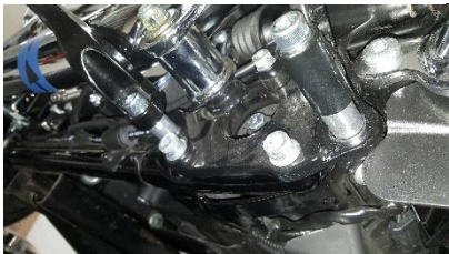
Figure 2.17 Install passenger peg.
