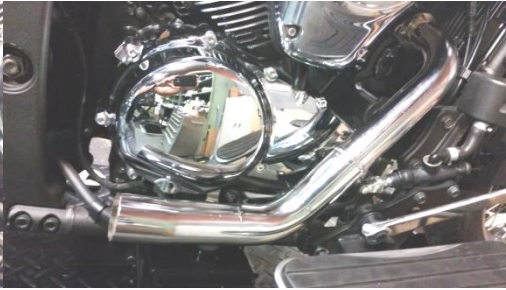
Figure 2.2 install front header use stock acorn nuts and M12 socket
