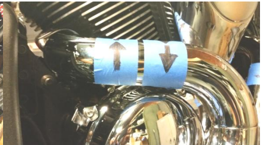
Figure 2.9 install rear shield section # 1 note: this shields sits on top of ring welded inside the other shield they must be flash
