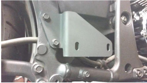
Figure 2.1 install bracket use stock screws and a M12 socket or wrench
