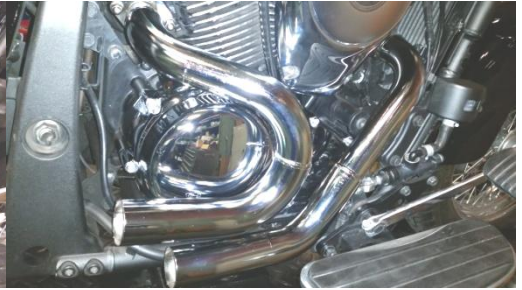
Figure 2.3 install rear header use stock acorn nuts and M12 socket
