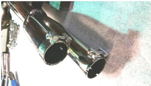
Figure 2.4 Install barrel clamps top screw faces up bottom faces down
