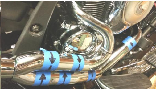
Figure 2.8 install front shield first then rear shield as shown
