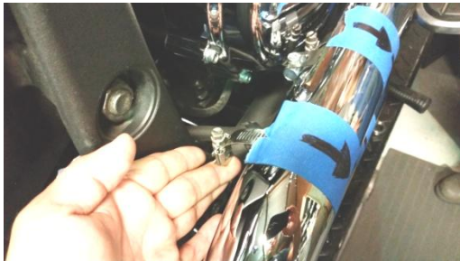
Figure 2.7 insert clamps as shown
