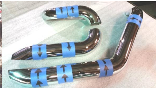
Figure 2.6 install painter tape and mark center as shown direction of arrow indicates hose clamp insertion
