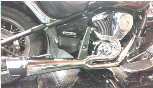
Figure 2.5 install muffler assembly use carriage bolts and flange nuts
