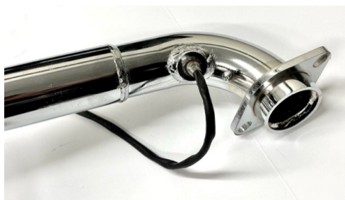
Fig. 2.2 install O2 sensor rear pipe
