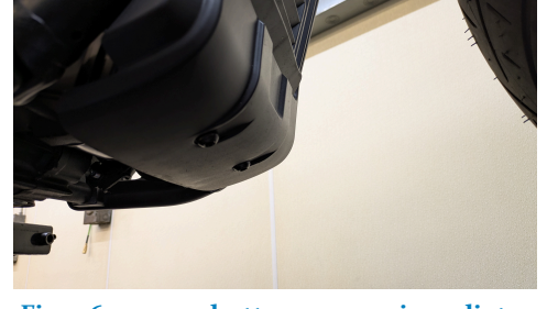
Fig. 1.6 remove bottom screws in radiator
