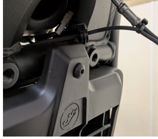
Fig. 1.5 remove top screw in radiator cover
