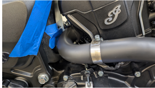
Fig. 2.5 insert clamp over inlets
