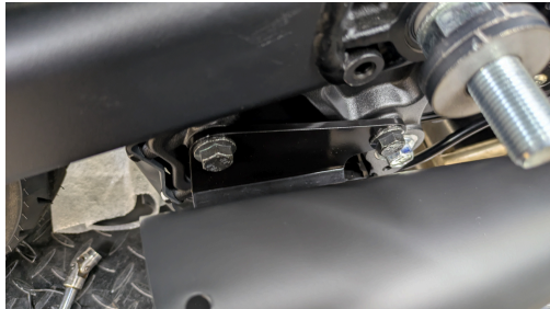
Fig. 2.4 install mounting bracket
