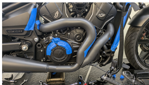
Fig. 2.8 install left and right header heat shield
