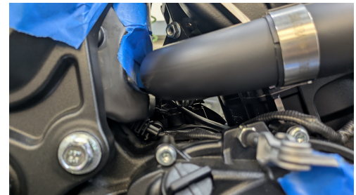
Fig. 2.3 install rear pipe
