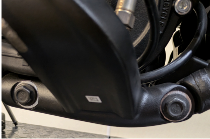
Fig. 2.15 reinstall foot controls
