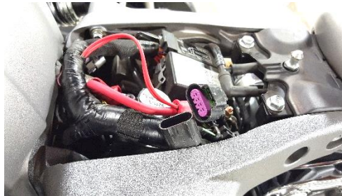
Fig. 2.15 reconnect O2 sensor plug back in
