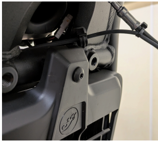
Fig. 2.13 reinstall radiator cover
