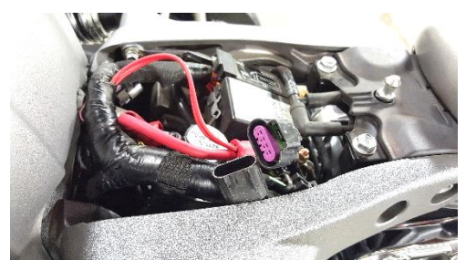
Fig. 1.3 disengage sensor harness
