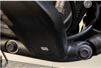
Fig. 1.7 remove foot control
