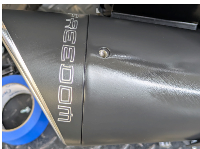
Fig. 2.10 install End cap with baffle attached
