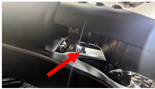
Fig. 1.2 loosen muffler clamp
