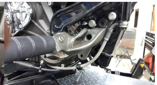
Fig. 2.20 install right control
