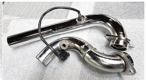
Fig. 2.2 install O2 sensor front pipe
