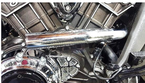
Fig. 2.3 install front pipe
