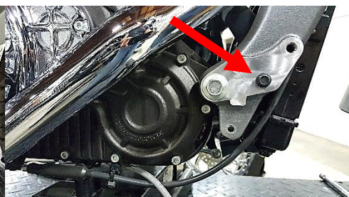
Fig. 1.14 remove screw right side
