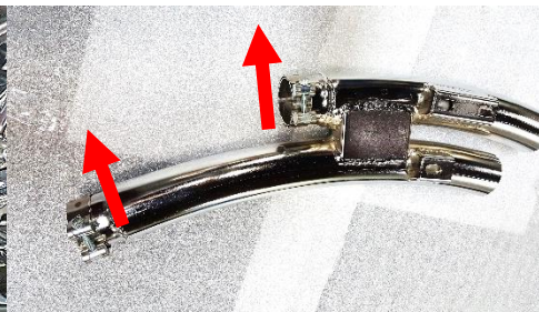
Fig. 2.7 insert clamps over inlets
