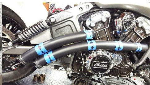
Fig. 2.16 install shields over
