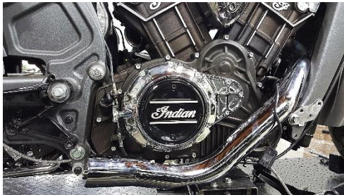
Fig. 1.22 remove rear pipe assembly
