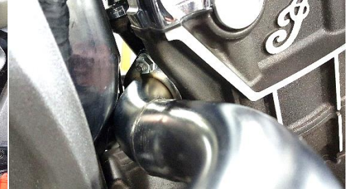
Fig. 2.11 tighten upper flange nut
