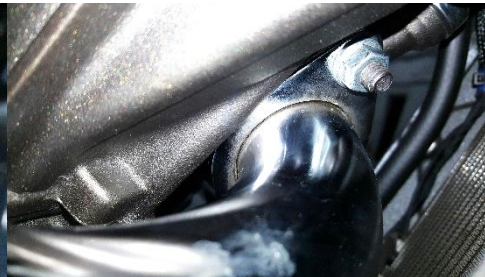
Fig. 2.13 tighten upper flange nut
