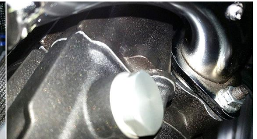
Fig. 2.14 tighten lower flange nut
