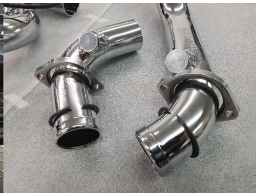
Figure 2.2 Install mounting bracket as shown. Figure 2.3 Install retaining rings & flanges/ install plugs (95-06) (09-16)
