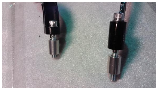
Figure 2.19 spacers shown for (09-16) models.
