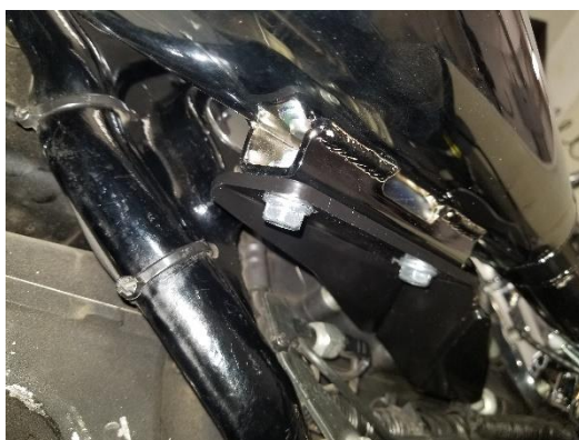
Figure 2.12 attach bracket to mounting bracket flush or a (+/-) 1/8"
