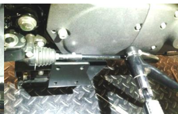
Fig. 2.2 picture may be different but same process, bottom screw engages both cover & bracket
