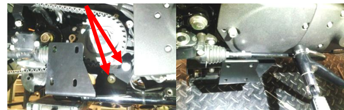
Fig. 2.1 install bracket picture may be different but same process use two stock screws
