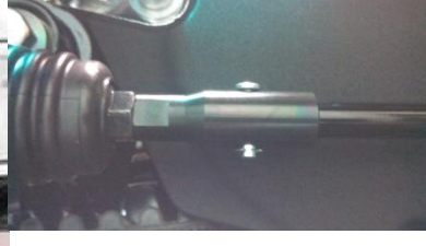
Fig. 2.4 (14-up) re-install pin
