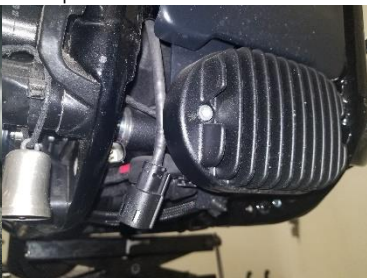
Fig. 2.8 disconnect front sensor
