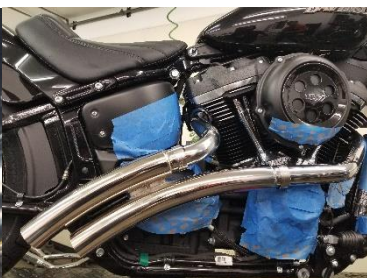
Fig. 5.15 install muffler assembly
