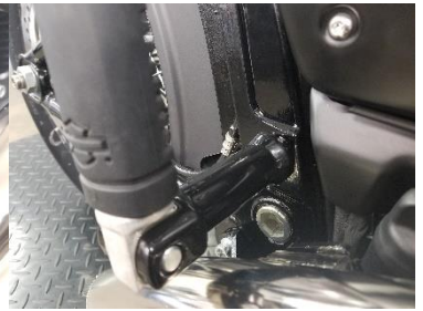
Fig. 5.24 reinstall peg on bracket.
