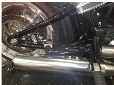
Fig. 3.10 remove mounting bracket
