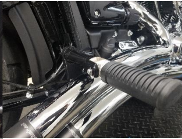
Fig. 5.27 install peg right side
