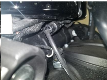
Fig. 2.7 disconnect rear sensor
