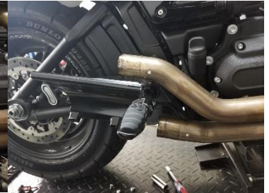
Fig. 1.8 remove lower muffler
