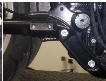
Fig. 1.19 remove mounting bracket
