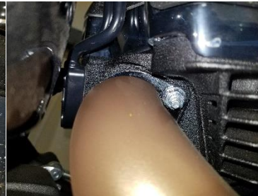
Fig. 1.11 remove rear flange nuts
