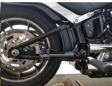
Fig. 3.5 remove lower muffler
