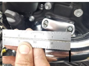
Fig. 5.14 mark a line @ 1-3/8" (35mm)
