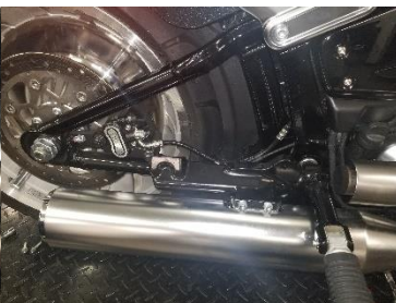
Fig. 3.9 remove front flange nuts
