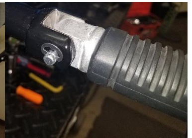
Fig. 1.16 remove retaining ring
