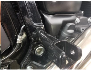
Fig. 5.23 install peg bracket
