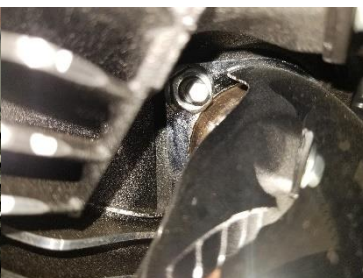
Fig. 3.9 remove front flange nuts
