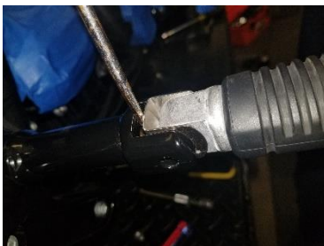
Fig. 1.17 pull pin and remove peg
