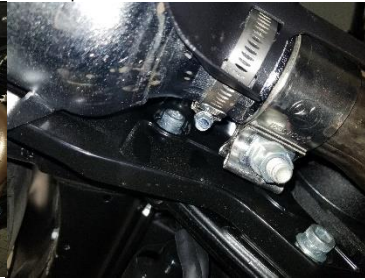
Fig. 1.3 remove hose clamps
