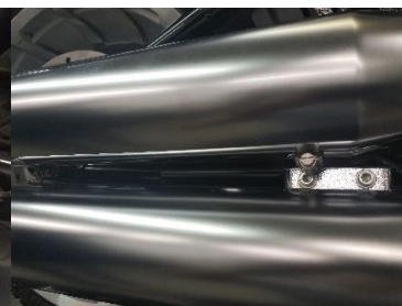
Fig. 2.4 remove lower muffler screws
