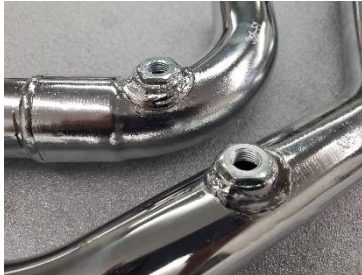
Fig. 5.9 install sensors adapters
