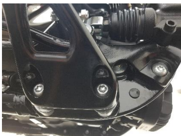
Fig. 3.6 remove mid control screws
