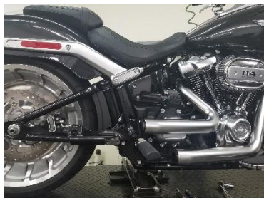
Fig. 2.6 remove lower muffler
