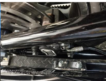
Fig. 3.1 remove upper muffler screws
