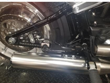
Fig. 3.8 remove rear flange nuts
