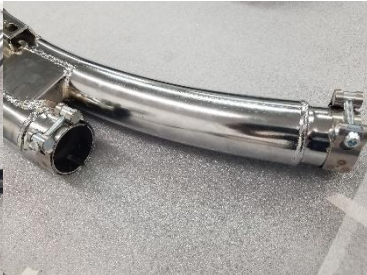
Fig. 5.11 insert barrel band clamps
