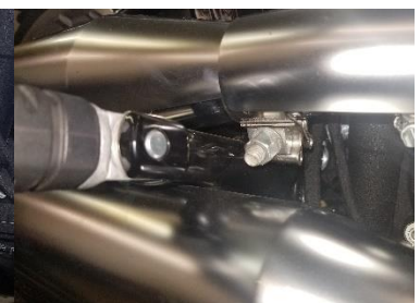
Fig. 2.1 loosen upper clamp
