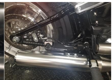
Fig. 2.5 remove upper muffler
