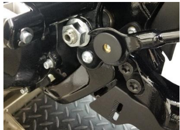
Fig. 5.29 saddle bag relocater bracket
