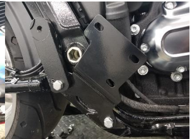
Fig. 5.4 wide tire right peg relocater
