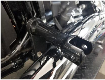
Fig. 5.25 wide tire bracket installation on right side
