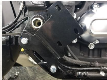
Fig. 5.2 install bracket wide tire
