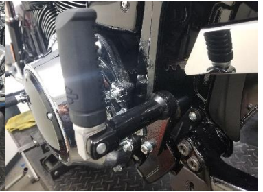
Fig. 5.28 install peg left side
