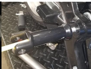
Fig. 1.18 remove peg bracket
