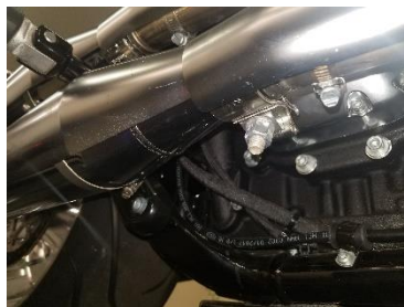
Fig.2.1 loosen lower clamp
