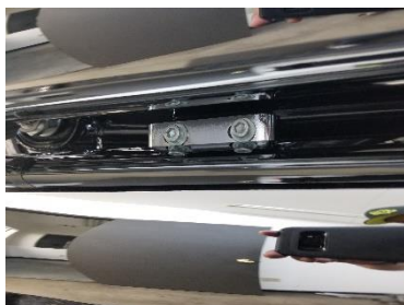
Fig. 3.2 remove lower muffler screws
