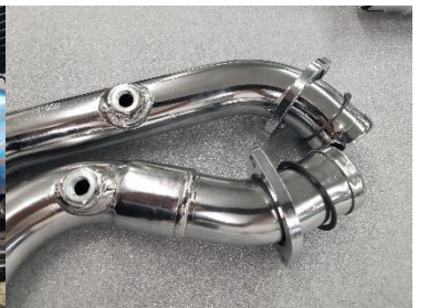
Fig. 5.8 install rings and flanges
