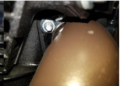
Fig. 1.12 remove front flange nuts
