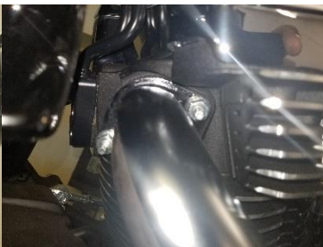
Fig. 2.9 remove rear flange nuts
