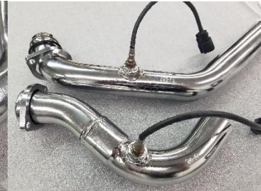
Fig. 5.10 install Oxygen sensors
