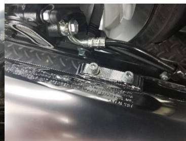
Fig. 2.3 remove screws upper muffler
