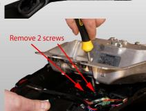
Remove screws to split fender
