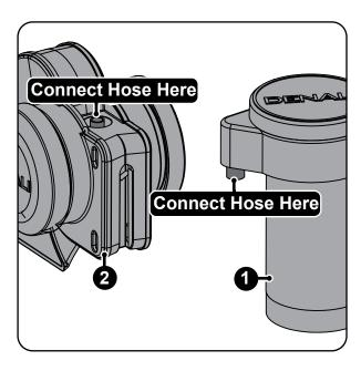
**Compressor Mounting:** Use the M8 bolt (#4) and nut (#5) to secure the compressor to you motorcycle. The compressor should be mounted so that the cylinder is vertical with no more than a 25 degree variance from the vertical position.
