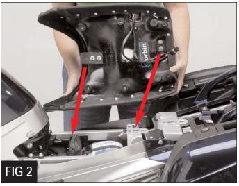
**NOTE:** If you have the rear rack / top case mount (#1MC-F48DO-V0-00), used for the 50 Liter Top Case, you will need to add spacers to the Smugglers rear bracket and rear rubber bumpers. Remove the bracket and place 2 spacers under each side of the bracket and secure with the provided 1/4 x 20 button head Allen bolts. Remove the bumpers and place 2 spacers under each bumper and secure with the provided 8/32 x 3/4 button head Allen bolts. (Figure 4)
