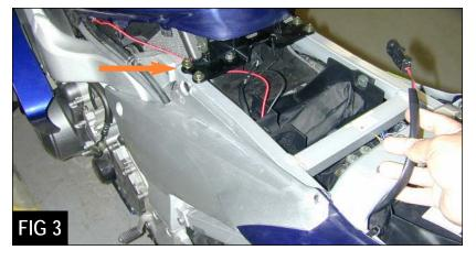
6. Before reinstalling the panel back in place, lay your seat on the bike and connect the plug to your seat heater. Turn on your ignition switch and test the seat. If the switch illuminates in both high and low positions, your saddle heater is working properly. Once it checks out ok, go ahead and resecure the fuse panel and your side panel back in place.
