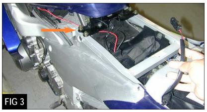
**NOTE:** The fuse box door will no longer close due to the pig tail being in the way so we have provided a fuse box rain cover.
